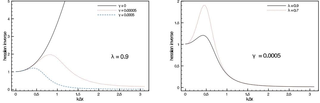
**Figure 1.** The inverse of the hessian,  $|\widetilde{\mathcal{H}}^{-1}(k)|$ , according to  $k\Delta x$  for different values of  $\gamma$  to the left and different values of  $\lambda$  to the right.
