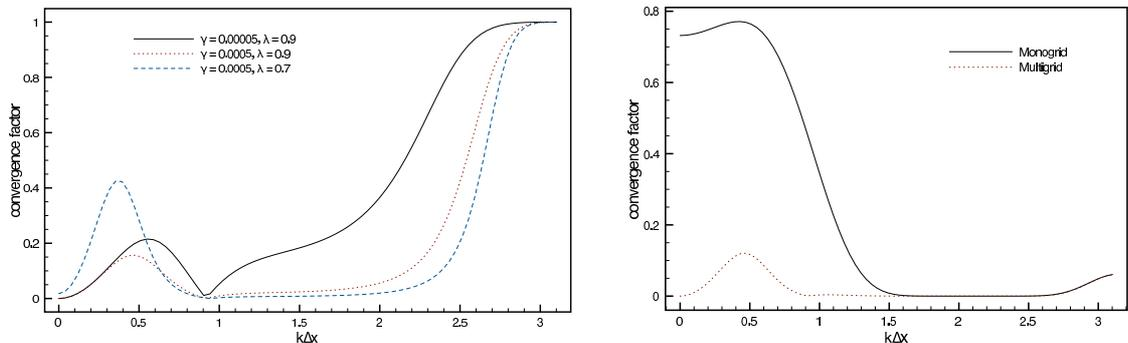
**Figure 2.** To the left, the convergence factor for one coarse grid correction according to  $k\Delta x$ , for different values of  $\gamma$  and  $\lambda$ . To the right, the convergence factor for the weighted-Jacobi on  $\Omega^f$  and for the multigrids using the same relaxation method on fine grid.
