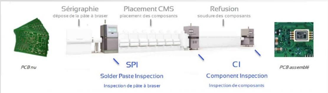
Printed Card Board assembly line.
