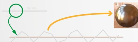
In this model, the surface micro-geometry is made of micro-facets, and that we have a probability distribution function describing the orientation of their normals. We can then express the overall material reflectance as an integral of the micro-facet reflectance multiplied this probability distribution.
