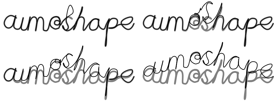
Fig. 5. Modification of a B-spline curve at various resolutions. A vertical select-and-drag operation at the top of the 's' character at four different resolutions. The original curve is presented in gray.
