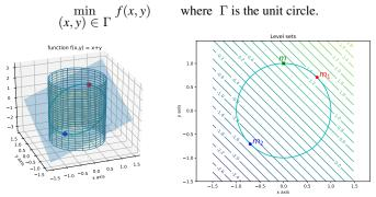
• 3D analysis : the objective function defines a plane and the constraint a circular cylinder, so that we are looking for the extrema of the 3D intersection curve of these two surfaces in the 3D space. • However, in practice, the analysis of this optimization problem will be based on 2D tools, and essentially on the level sets of the objective function, which are here straight lines.
