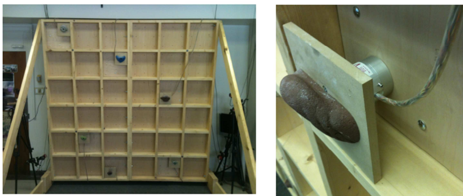
Figure 1. – Climbing wall equipped with force sensors
