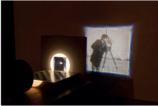
Figure 20. Lens transforming collimated light into the picture of a cameraman
