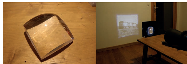
Figure 19. Lens transforming collimated light into the picture of a train
