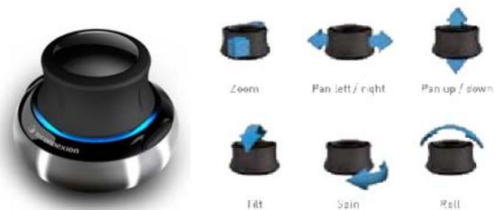
Figure 3. The SpaceNavigator and its degrees of freedom.
