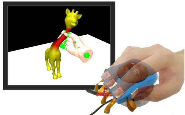
Figure 1. HandNavigator: hands-on interaction peripheral device for virtual reality and applied to the manipulation of deformable objects.
