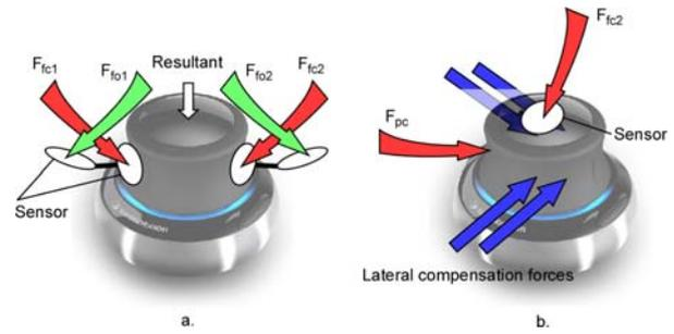
Figure 6. Force compensation (here with two fingers). In red: closing pressure ( $F_{fc}$  for the fingers and  $F_{pc}$  for the palm), in green: opening pressure ( $F_{io}$  for the fingers), in blue: compensation forces. a.: homogeneous distribution of forces when opening/closing simultaneously two fingers. b.: if the sensor is on the top of the device, it is necessary to apply strong lateral forces to maintain the desired wrist configuration.
