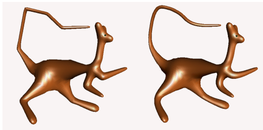
Figure 1. From [6]: an implicit object defined from a graph of subdivision curves with two different LODs.
