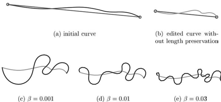
**Fig. 1.** Role of  $\beta$ : the initial curve (a) with 129 control points is edited at the coarsest level (b) (in gray: reconstructed attracting curve). In (c), (d) and (e): 3 final length preserving curves (in black) are given for different values of  $\beta$
